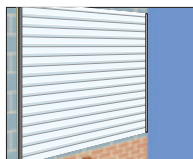
Fit remaining planks and engage male part of two-part trims.
