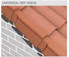
The Marley Universal Dry Verge system has been designed to make verge detailing secure, BS 5534 compliant and elegantly simple.
