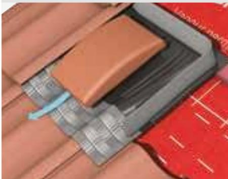
Suitable for roof void ventilation and connection to 110mm soil/mechanical extraction. Compatible with large format interlocking tiles and roof pitches 20° and above.
