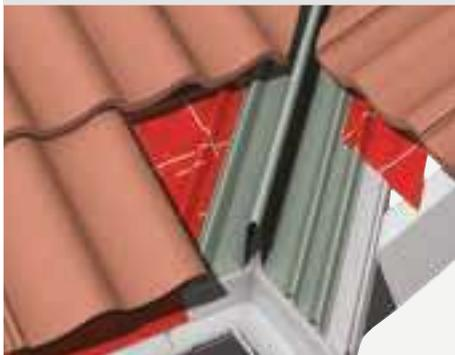
Mortar-free solution suitable for use with concrete interlocking tiles and concrete/clay plain tiles. Suitable on rafter pitches from 17.5-60° and accommodates up to 20° pitch difference either side of valley.
