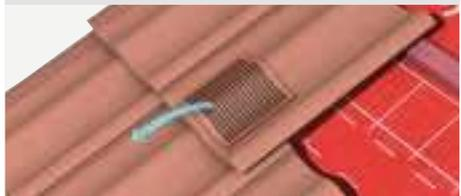
Discreet high performance vent terminals for high/low level roof space ventilation. Suitable for soil and mechanical ventilation. Minimum roof pitch 22.5° (except Plain tiles 35°).
