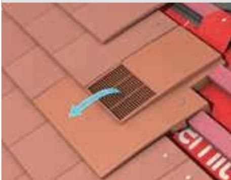
Designed for natural, mechanical or soil pipe ventilation. Provides 10,000mm<sup>2</sup> free area of ventilation and suitable for concrete and clay plain tile roof pitches 22.5° and above‡.
