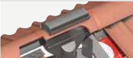
Suitable for natural soil, or mechanical ventilation. Provides high level ventilation for concrete tiles (9,500mm<sup>2</sup> free area), clay plain tiles (10,000mm<sup>2</sup> free area).
